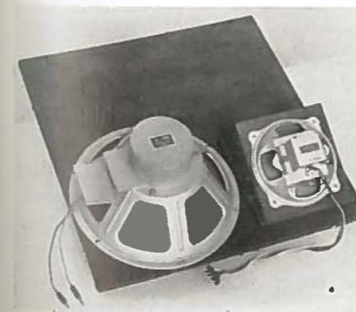
Fig. 4 X 4480 Baffle with loud-speakers The larger one, with a cone area of 600 cm 2 , reproduces the bass register, the smaller one the top register
