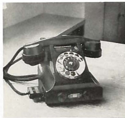
Fig. 1 Telephone instrument with built in signal lamps for connection to the amplifier, Fig. 2
