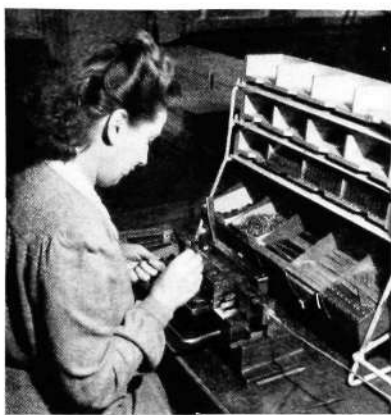
Fig. 13 X 4632 Mounting contact spring layers on vertical unit base
