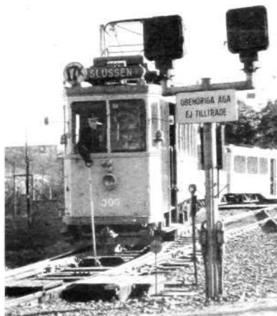
Fig. 3 X 4624 The driver transmits impulse to the interlocking machine by means of the pedal contact
