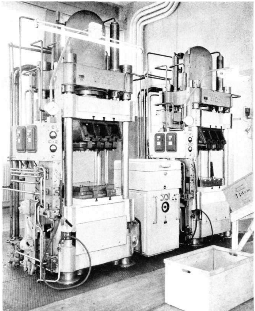
Fig. 6 200/100 ton presses working together with a high frequency unit
