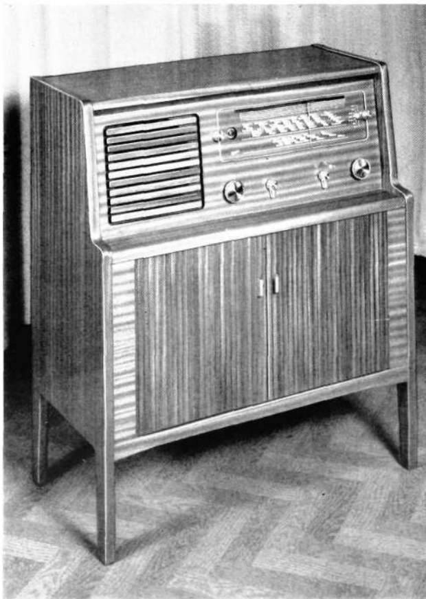
Fig. 3 X 7624 Ericsson Pianett left: with roller shutters closed. The controls are from left to right: volume control, tone control, off-on, radio-phone-switch control, combined tuning- and wave-band switch.
