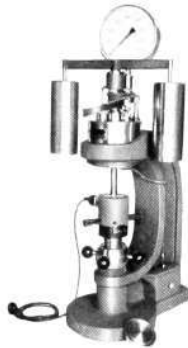
The smaller picture shows a modern Brinell tester.
