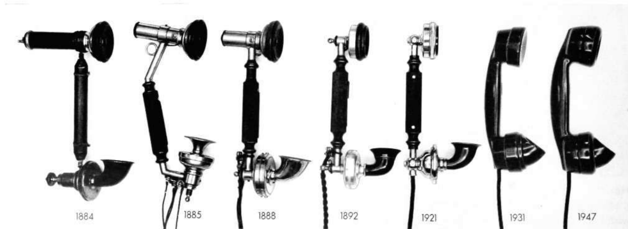
Fig. 9 X 7634 The main outlines of the development of the L M Ericsson handset from 1884 to 1947
