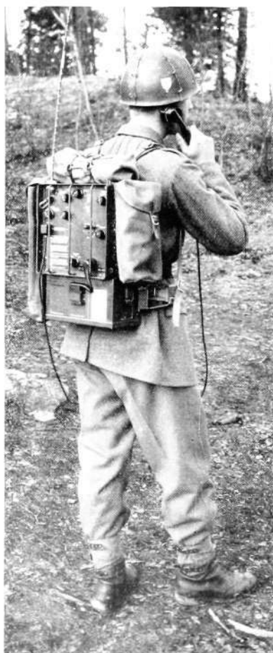
Fig. 1 X 4745 Portable field radio equipment SUF-21 K
