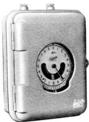
Fig. 3 X 4773 Indicating receiver KCT 2011—KCT 2017 for different impulse intervals and ranges
