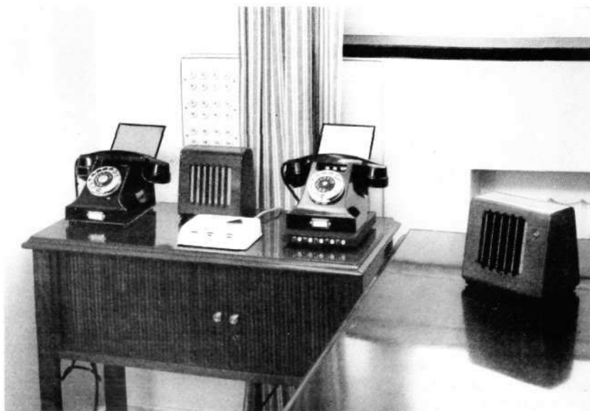
Fig. 6 X 6670 Master instrument for conference tele- phone system with extension unit for 5 extensions and equipment for loud speaking telephone. In the centre the white desk panel and the wall lamp panel for attendance indication.
