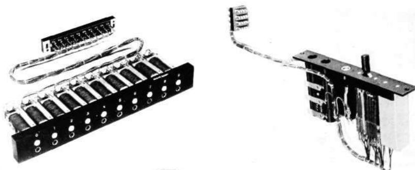
Fig. 18 X 4855 X 4856 Connecting elements for manual switchboards ADE and ADF left line unit, right switching set.
