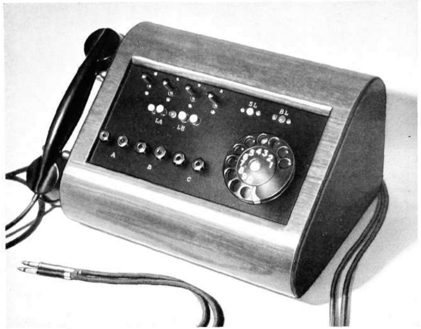
Fig. 3 X 6732 Test set for checking individual connection stages in a decimal by-path system
