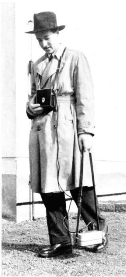
Fig. 19 X 4971 Radiation intensity meter LMK 3001 in use
