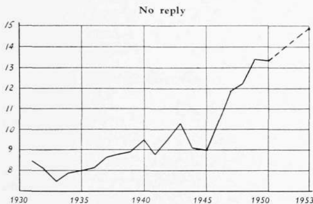
Fig. 2 X 6901 X 6902 Percentage of «no faults» for Stockholm central area exchanges, divided in main groups according to table 2, during the period 1930—1953
