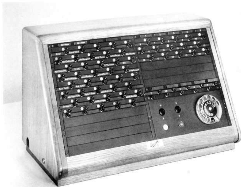
Fig. 2 X 6788 Operator's direction set for semi-automatic call distribution at the booking office for sleeping car accommodation, Swedish State Railways in Stockholm
