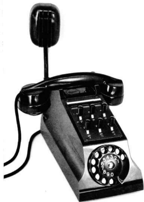
Fig. 1 X 4962 Cordless switchboard ADD 1311 for 3 extensions and 1 public exchange line
