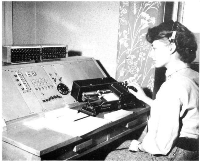
Fig. 2 Equipment for traffic observations (random checks) Helsinki Telephone Corporation, the traffic bureau
