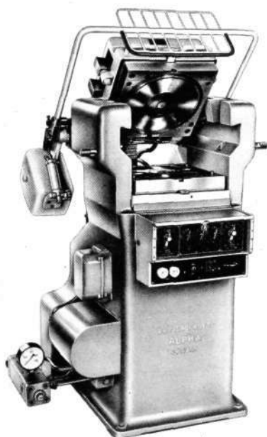
Fig. 6 ALPHA gramophone record press
