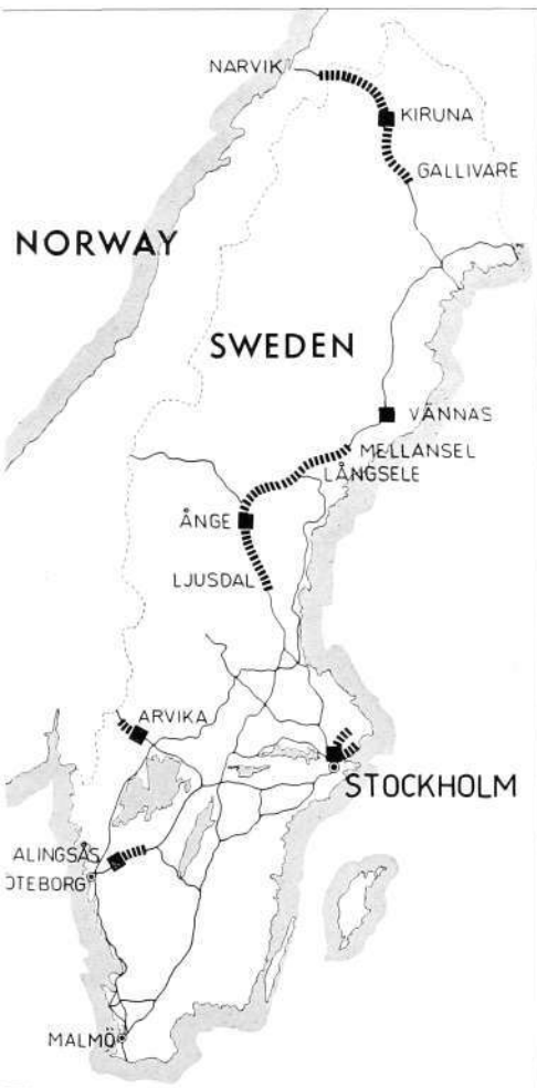
Fig. 7 X 2533 X 9151 C.T.C. plants of the Swedish Railways installed and scheduled. All plants have been or will be delivered by L M Ericsson.
