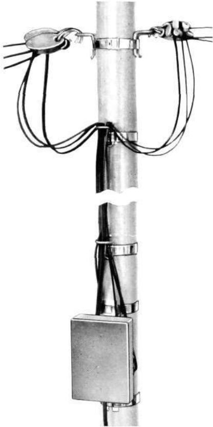
Fig. 1 The new distribution box on a tubular steel pole
