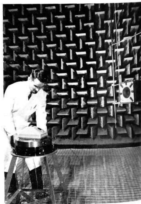
Measurements on the Ericovox loudspeaking telephone in the "quiet room".
