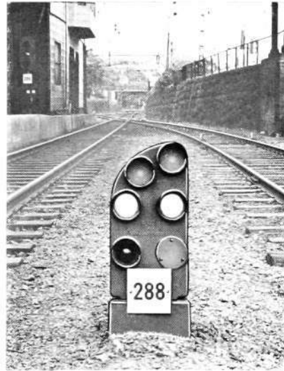
Fig. 3 Position-light shunt signal with four white apertures and one green
