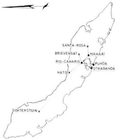
Fig. 2 Curaçao's telephone network ● Local exchange ● Satellite exchange
