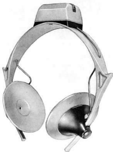
Fig. 2 Headset RLD 9811 with transistor receiver for magnetic loop
