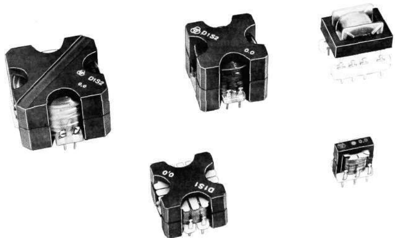
Fig. 7 Ferrite cored transformers of different sizes: Top row from left—mounting height 23.5 mm: REG 302 (X 36), REG 301 (X 30), REG 203 (E 25) Bottom row from left—mounting height 15.5 mm: REG 316 (X 25), REG 204 (E 14.5)
