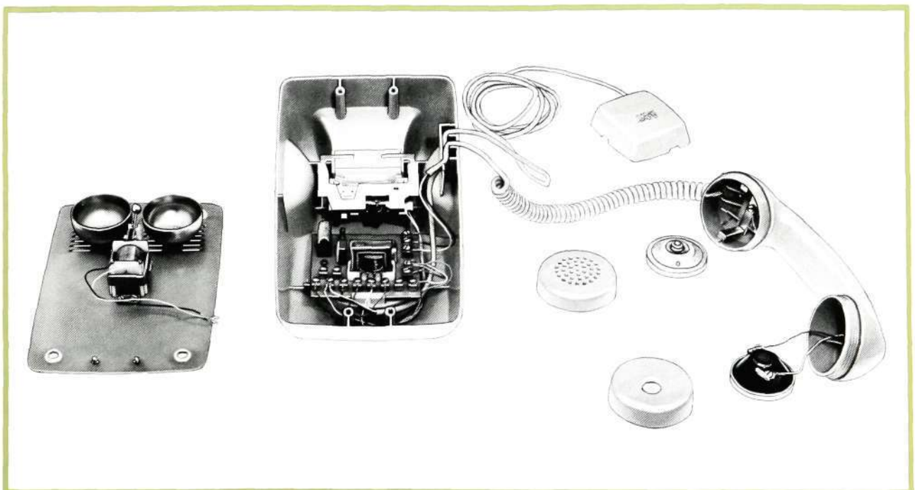
Fig. 3 Simple mechanical design facilitates servicing
