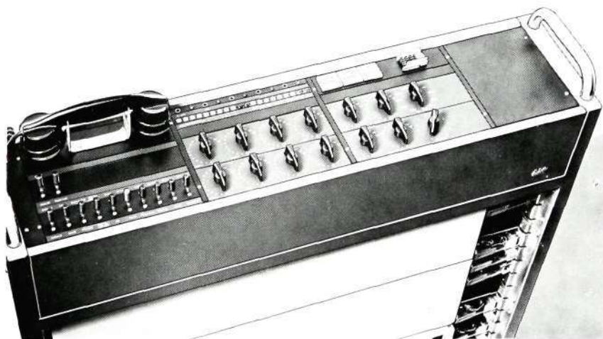
Fig. 7 (right) Fault tracing with SL-GV tester
