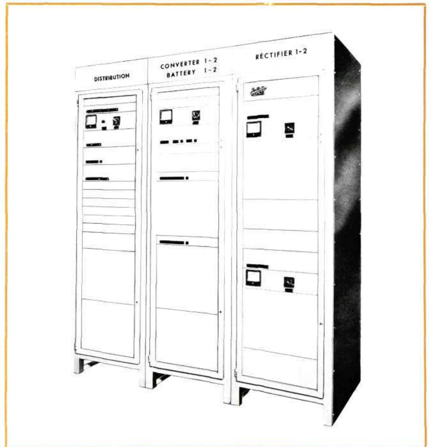
Fig. 10 Power supply plant 48 V with two non-regulated booster converters 100 A, two rectifiers 100 A and distribution bay. The distribution bay contains control and supervisory units and fuses for outgoing cables.
