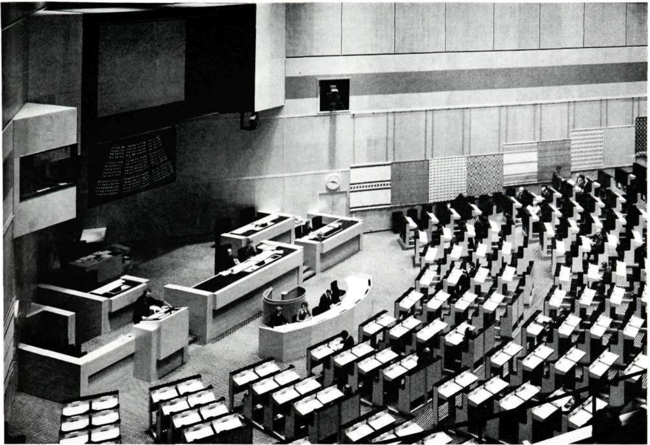
Fig. 1 Plenary chamber viewed from visitors' gallery. (Left) Control room, in the rear above the podium the 3.5×4.5 m projector screen, thereunder the voting panel and the moving TV cameras.
