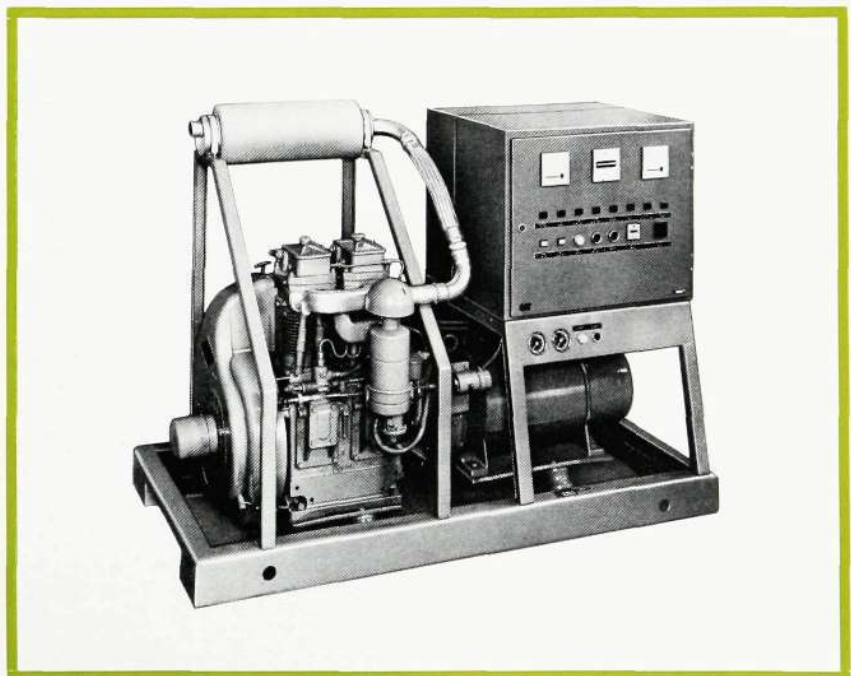
Fig. 7 Standby power unit 5 kVA at \cos \varphi = 0.8 , 220 V, 1-phase, 50 Hz, 1000 r.p.m. Engine: Petter PH 2 Generator: A. van Kaick WKB 30/3—6 TS
