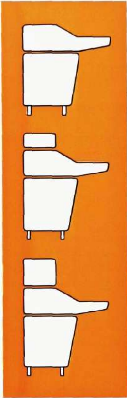
Fig. 4 Switchboard with sloping keyshelf. The middle figure shows a switchboard with low vertical panel added and the bottom figure with high vertical panel
