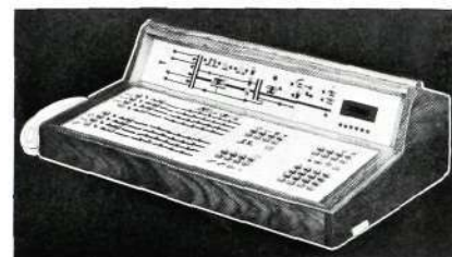
An operator's console for the new electronic exchange ASD 551.
