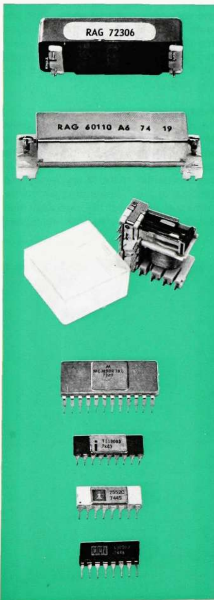
Fig. 14 Different types of miniature relays (top) and memory components (below) used in ARE 13
