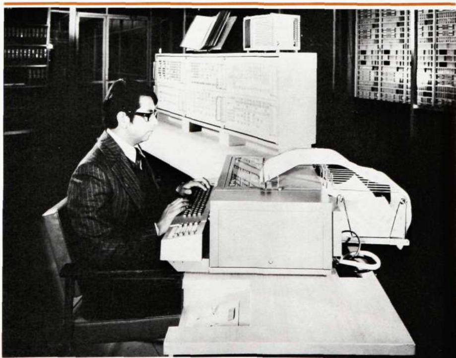
Fig. 5 Control room in San Juan with typewriter, for communication between service staff and the plant, and the control panel for the processors
