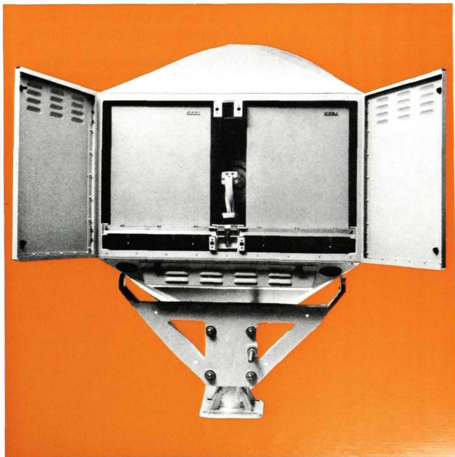
Fig. 10 The radio-relay equipment with the protective cover removed. The upper illustration shows the equipment from the front and the lower from the rear
