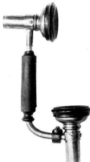
R 302 Fig. 2. Trial Model with two Receivers.
