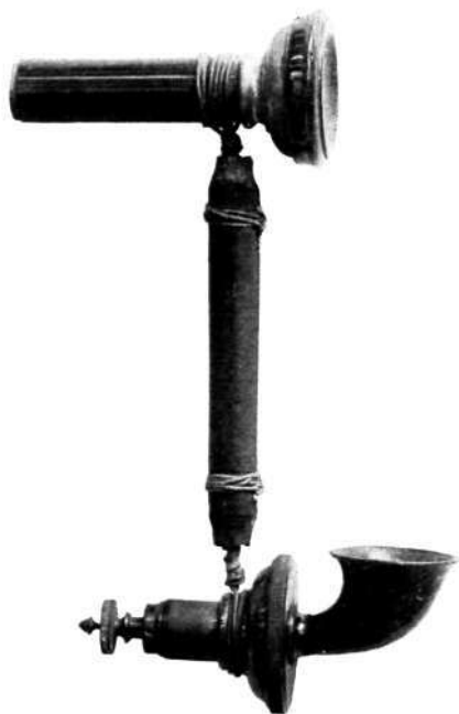
R 303 Fig. 1. The First Hand Micro-telephone.
