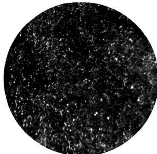
Magnet Steel. 6 % Tungsten. Unspoiled. 800 diameters.
