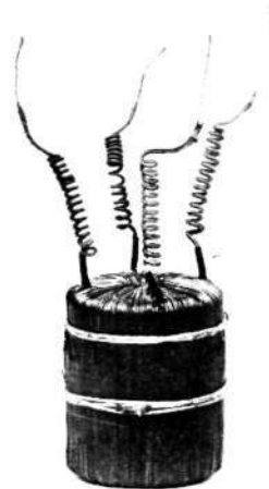
Transformer, with case removed.
