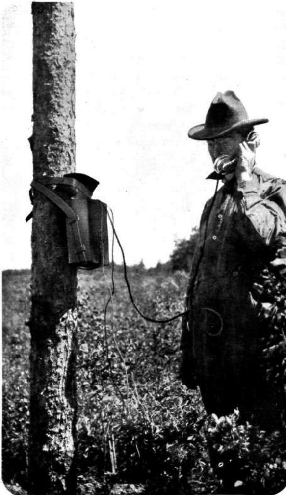
R 897 Portable Telephone for use in Trouble Finding on Fire Alarm Telephone Lines. Canada. (Foto. Can. Forest Service.)
