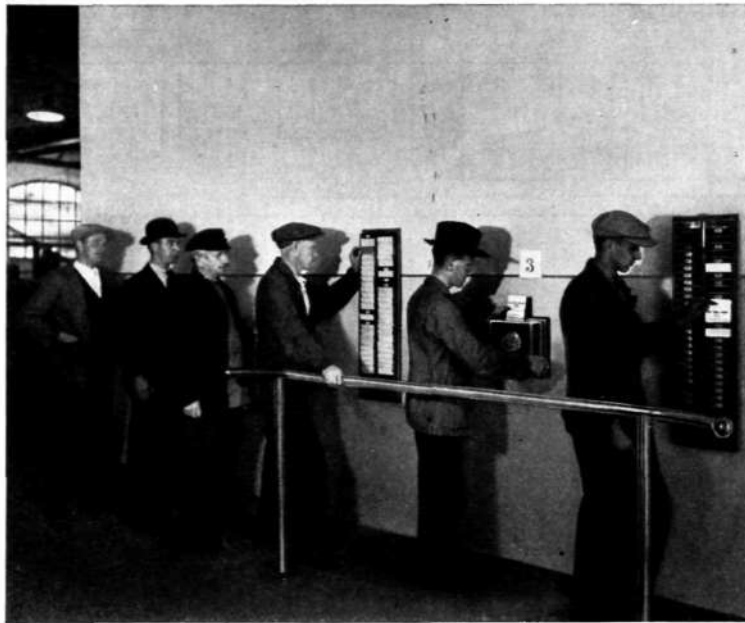
R 786 Time Recorder and Card Files for Registration of Times of Arrival and Departure.
