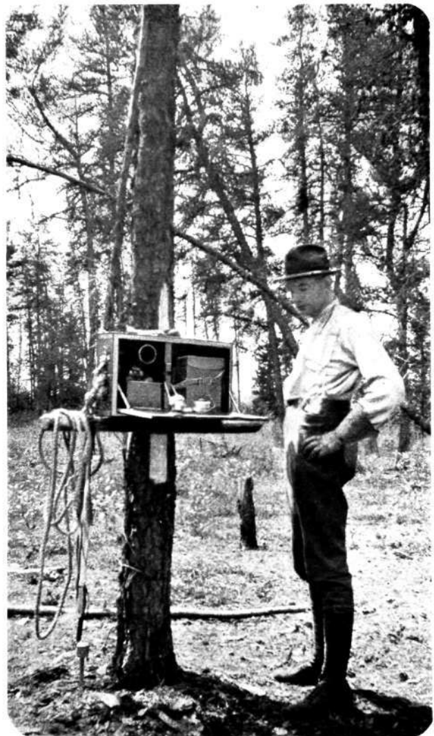
R 889 Canadian Forest Service Emergency Communication Kit in Use. The set contains in the smaller compartment 1 extension bell, 1 protector, 1 howler, 1 condenser. The larger compartment is fitted with 2 binding posts, from which wires lead to the external connections in the set and a portable telephone. There is also room for tools, etc.
