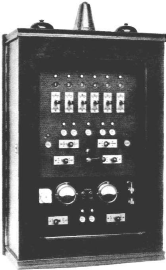
Fig. 2. An Automatic Fire Alarm Station Apparatus for 6 Sections, including Charging Board for Storage Batteries. The diagram shows signal lamps and various illuminated signs which, together with bells, automatically register fire alarm and faults of every kind, and also control that every switch is correctly thrown.
