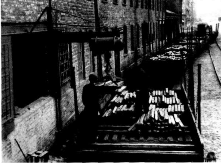
R 3088 Unloading copper billets at the mill from a railway truck.
