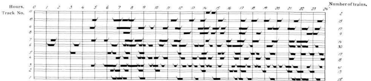
Fig. 4 a. Occupation of the platform tracks according to the time table 1930-31.
