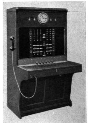
Fig. 6. Switchboard at the police station. The apparatus is composed of units acc. to Fig. 8, connected to one line each.
