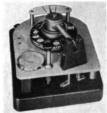
x 3092 Fig. 1. The ratio tester with the dial in place for the test.
