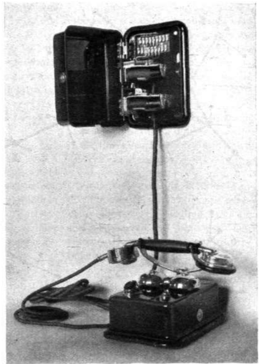
Fig. 2. Selective calling telephone instrument, for connection to LB or CB systems
