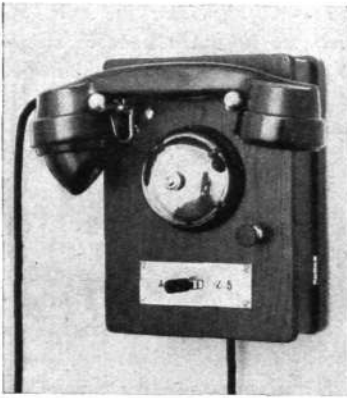
X 3074 Fig. 4. Instrument for use in well sheltered places, e. g., the engineers cabin.
