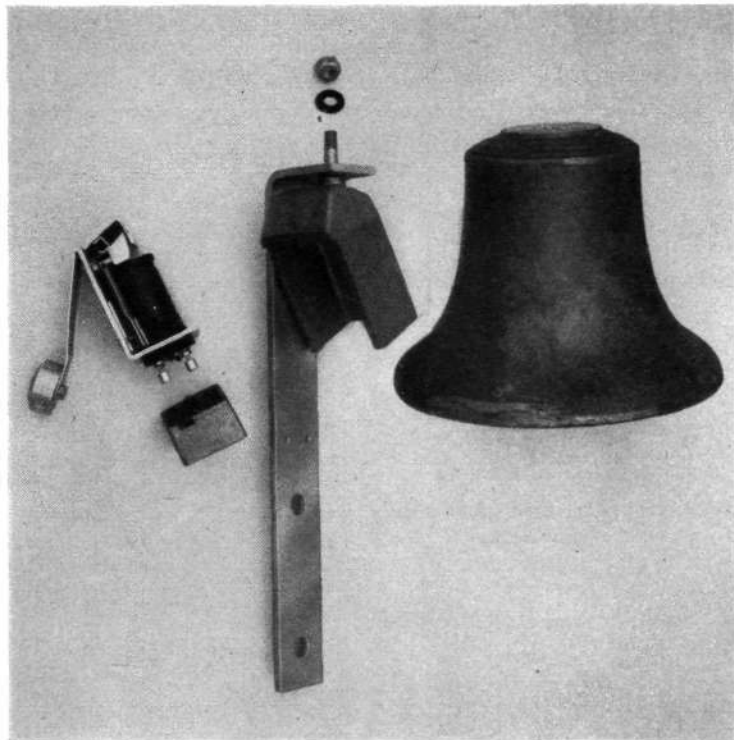
Fig. 7. Alarm bell, dismantled.
