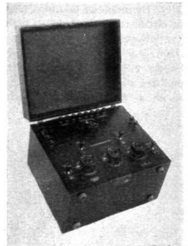
X 3111 Fig. 7. Cross-talk meter, Type ZB 256.
