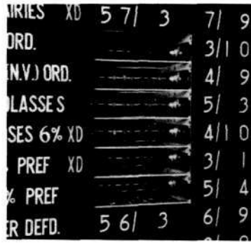
X 3278 Fig. 5. Detail of indicator board, showing the rotating driving shafts.
