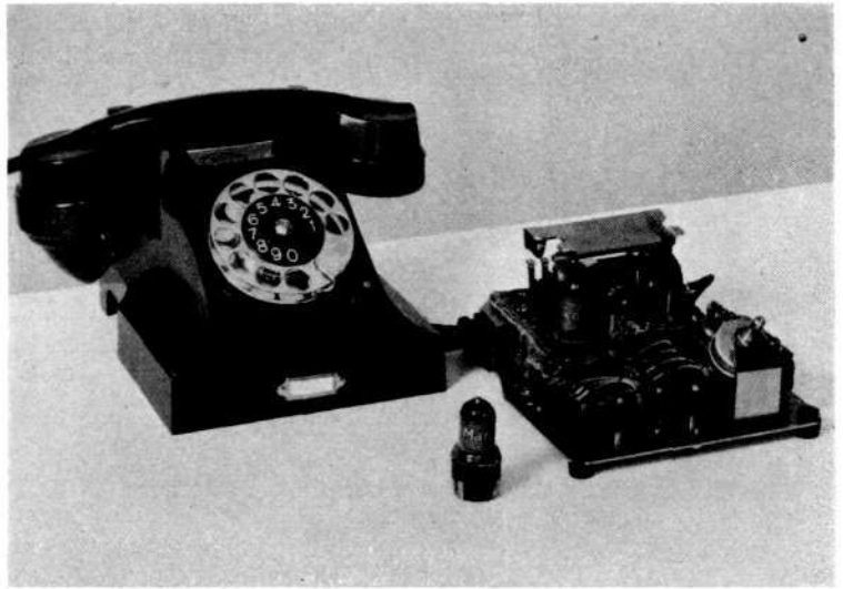
X 5172 Fig. 1. Telephone instrument with built-in amplifier. Left, instrument box with microtelephone, dial and volume control; middle, amplifier valve; right, inset with amplifier.
