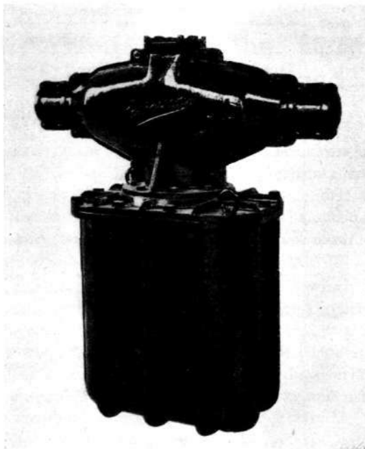
X 1350 Fig. 3. Loading-coil case containing 38 coils. The main cable is connected to the coil cable in the splicing box at the top.
