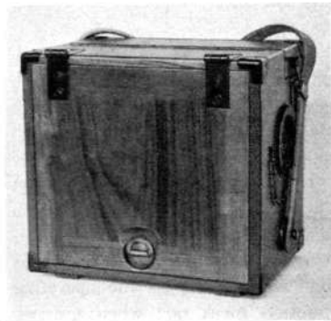
Fig. 8 6-line field telephone switchboard from Elektrisk Bureau, Oslo
