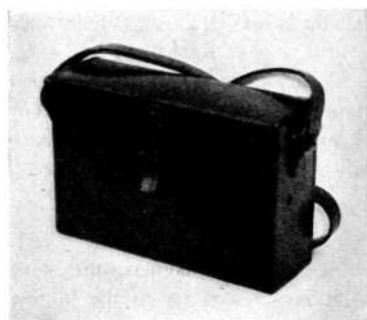
Fig. 1 Field telephone instrument in leather case
