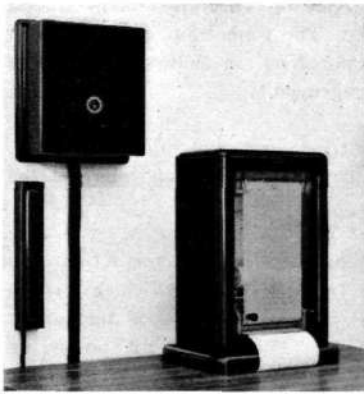
Fig. 1 Recording apparatus on wall, relay set
