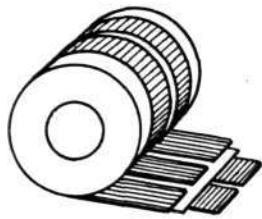
Fig. 1 Design of condenser element
