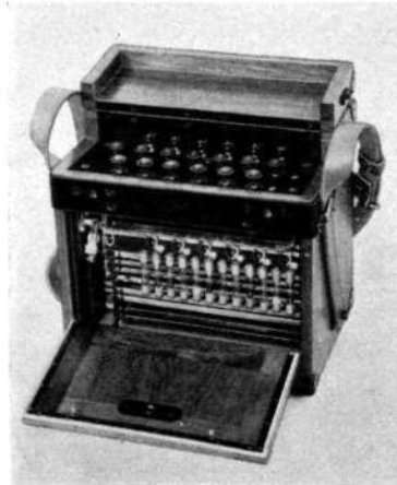
Fig. 9 - 6-line field telephone switchboard from Elektrisk Bureau, Oslo with back lid down for changing rare-gas tubes
