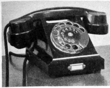
Fig. 1 Telephone instrument, Type DBK 11 all instruments are of normal pattern without push button and are connected over two-wire lines without additional wire or earth connection
